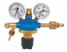
Standard pressure regulator (construction same as Art. 5100, but for inlet pressure up to 300 bar) with excellent pressure consistency. Equipped with pressure and contents gauges, integral safety valve and shut-off valve in the outlet.
