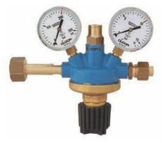
This pressure regulator has the same construction as Art. Nr. 5100 and is suitable as a central pressure regulator for small gas supply systems. Also available with working pressure up to 60 bar. With pipeaway facility fitted to safety valve for venting gases to atmosphere.
