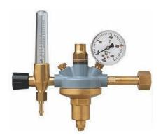
Pressure regulator with contents gauge and with built-on flowmeter. Integral safety valve and shut-off valve on flowmeter. The flowmeter design ensures a clear reading of the delivered flow rate. Accuracy of measurement of the flowmeter +/-10%. Available in three flow rates (see below).
