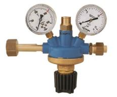
This pressure regulator has the same construction as Art. Nr. 5100 and is suitable as a central pressure regulator for small gas supply systems. Also available with working pressure up to 60 bar. With pipeaway facility fitted to safety valve for venting gases to atmosphere.
