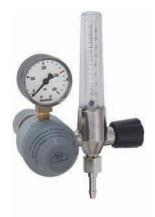
Pressure regulator with fitted flowmeter with fine regulation spindle (serves at the same time as shut-off valve) and safety valve. Accuracy of measurement of flowmeter +/-10%. Available for three different flow rates (see below).
