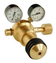
The pressure regulator is available in version for working pressure up to 100 bar or up to 200 bar. The working pressure is infinitely adjustable with the handwheel between 10-100 bar, resp. between 10-200 bar. For an easy pressure adjustment the handwheel shows at the front a hexagon, so that the pressure adjustment can also be made by means of a socket wrench 8 mm.
