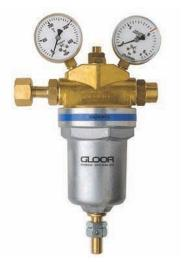
High flow rate pressure regulator (construction same as Art. 7900, but for inlet pressure up to 300 bar). With working pressure and contents gauges and integrated safety valve. Standard version with working pressure up to 10 bar. Also available with working pressure up to 20, resp. 30 bar (s.below).
