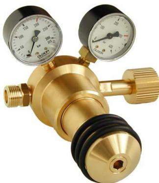
Pressure regulator for high working pressure up to 100, resp. 200 bar (construction same as Art. 7902, but for inlet pressure 300 bar). Piston pressure reducing valve which guarantees for a precise and stable setting of the secondary pressure.
