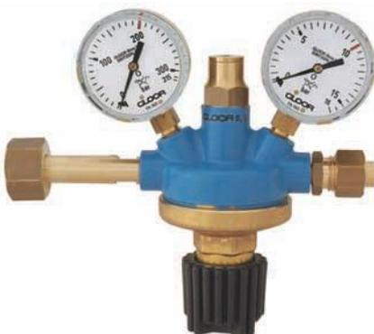
This pressure regulator has the same construction as Art. Nr. 5100 and is suitable as a central pressure regulator for small gas supply systems. Also available with working pressure up to 60 bar. With pipeaway facility fitted to safety valve for venting gases to atmosphere.
