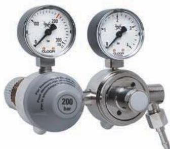
Two-stage pressure regulator with indication of cylinder content and working pressure. Particularly suitable for applications requiring a very constant secondary pressure. Working pressure preset from 0.5 to 3 bar (as required). Also available with Teflon coated diaphragm for analysis equipment.
