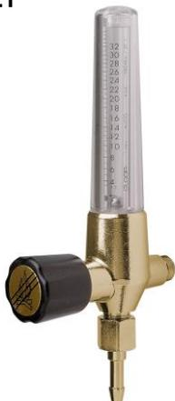
Flowmeter only, accuracy of measurement +/-10%, with shut-off valve. Calibrated to a preset inlet pressure of 4,5 bar; available for three flow rates: 0-3, 0-16 or 0-32 l/min.
