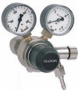
Pressure regulator with pressure and contents gauges, integral safety valve and shut-off valve in the outlet. Inlet at the rear, pressure adjusting screw at the front. Material: brass, nickel plated. Sintered filter in bronze, diaphragm made of Neoprene EFFBE.
