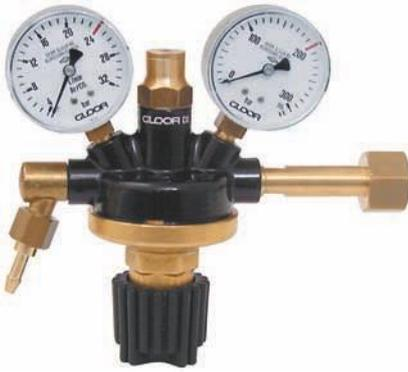
Pressure regulator with flow gauge, i.e. with indication l/min on secondary gauge. Integral safety valve. This pressure regulator is a cost effective alternative to Art.5150. With this system the flow is regulated by adjusting the secondary pressure (also via a throttle valve in the outlet).
