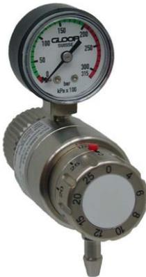
Very simple handling by setting of the desired flow-rate on the flow selector. High level of accuracy of measurement irrespective of the cylinder pressure. With integrated safety valve and gauge with indication of the cylinder pressure. The field of application is mainly in TIG, MIG, WIG and MAG welding.
