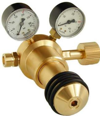
The pressure regulator is available in version for working pressure up to 100 bar or up to 200 bar. The working pressure is infinitely adjustable on the handwheel between 10 – 100 bar, resp. between 10 – 200 bar. For an easy pressure adjustment the handwheel shows at the front a hexagon, so that the pressure adjustment can also be made by means of a socket wrench 8 mm.
