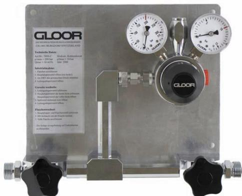
Manual change-over switching station for high purity gases with purity up to 6.0, consisting of two high pressure shut-off valves for alternate cylinder operation, main pressure regulator with safety valve, including purging valve. All parts fixed on an aluminium baseplate with specific gas identification.
