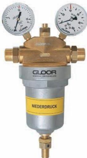
Low pressure regulator Type 79 for very high flow rates with an inlet pressure up to 40 bar. With working pressure gauge and adjusting screw for the precise regulation of the working pressure at the workplace.
