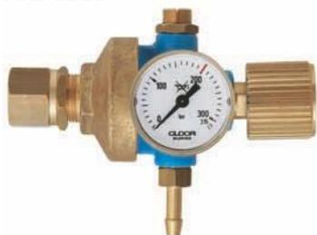
Pressure regulator with high pressure gauge (diameter 40 mm) for the indication of the cylinder content. With preset working pressure up to 8 bar (as required). Integral safety valve.
