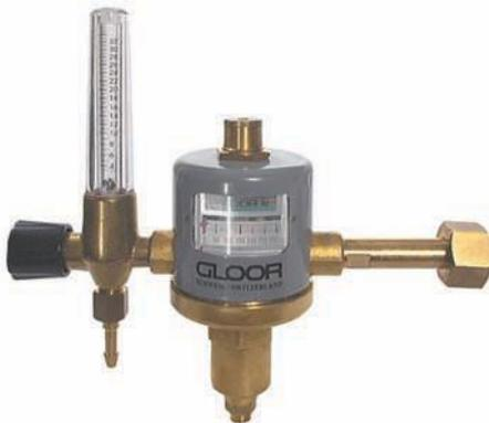
With fitted flowmeter and gauge showing cylinder contents. Integral safety valve and shut-off valve on flowmeter. Accuracy of measurement of flowmeter +/-10%. Available in three different flow rates (see below).
