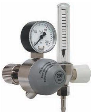
Pressure regulator with contents gauge and fitted flowmeter; integral safety valve. The flowmeter design ensures a clear reading of the delivered flow rate. Diaphragm made of Neoprene EFFBE; also available with Teflon coated diaphragm upon request.
