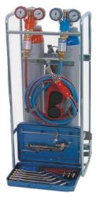
Complete portable welding and cutting outfit, including carrying frame with straps and belt for mounting a light steel cylinder of both oxygen and acetylene with diameter 100mm, two mini pressure regulators, two flame arrestors, complete light welding and cutting equipment in metal box, hoses, welding goggles and gas lighter.
