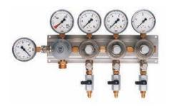
Combinded high / low pressure reducing station in monoblock design. Pressure regulator in brass, nickel plated. Covered pressure adjusting screw. Sintered filter made of bronze, diaphragm made of Neoprene EFFBE. Low pressure gauge with scale division 1/10 bar, as option 0-4, 0–6 or 0–10 bar, and with corresponding markings at 3, 4 or 7 bar.
