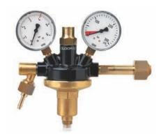
High pressure regulator with cylinder connection and/or with wall bracket for connection of high pressure hose. Alternatively for carbon dioxide, nitrogen or mixed gas. Contents gauge with red marking, working pressure gauge with scale division 1/10 and marking of the adjusted maximum pressure at 3, 4 or 7 bar.
