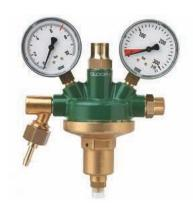
High pressure regulator with wall bracket for direct connection of the high pressure hose. Alternatively for carbon dioxide, nitrogen or mixed gas. Contents gauge with red marking, working pressure gauge with scale division 1/10 and marking of the adjusted maximum pressure at 3, 4 or 7 bar.
