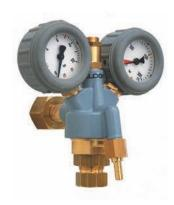
High pressure regulator with cylinder connection. Alternatively for carbon dioxide, nitrogen or mixed gas. Contents gauge with red marking, working pressure gauge with marking of the adjusted maximum pressure at 7 bar.
