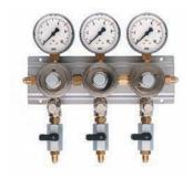
Low pressure regulator, made of brass, nickel plated. Covered arrangement of pressure adjusting screw. Sintered filter made of bronze, diaphragm made of Neoprene EFFBE. Low pressure gauge with scale division 1/10 bar, as option 0–4, 0–6 or 0–10 bar, and with corresponding markings at 3, 4 or 7 bar.
